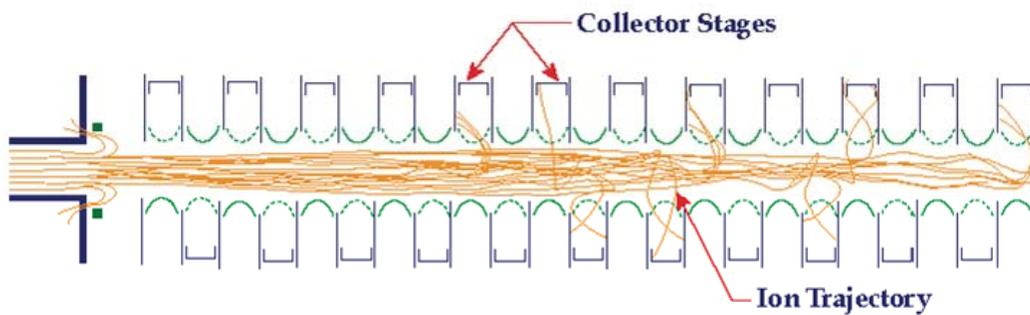
A 22-stage PDC with ion trajectories inside focusing and collecting system.\*
