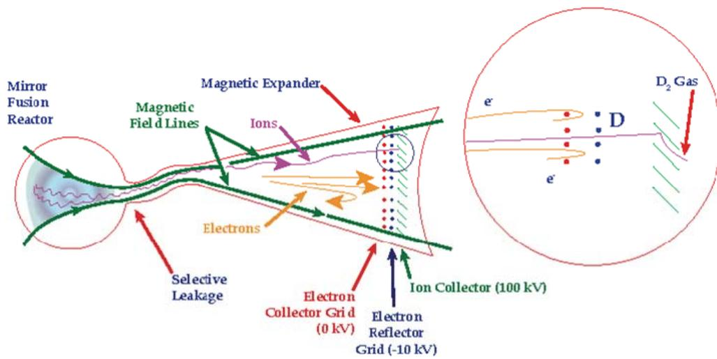
A simple one-stage PDC with conical magnetic expander.\*
