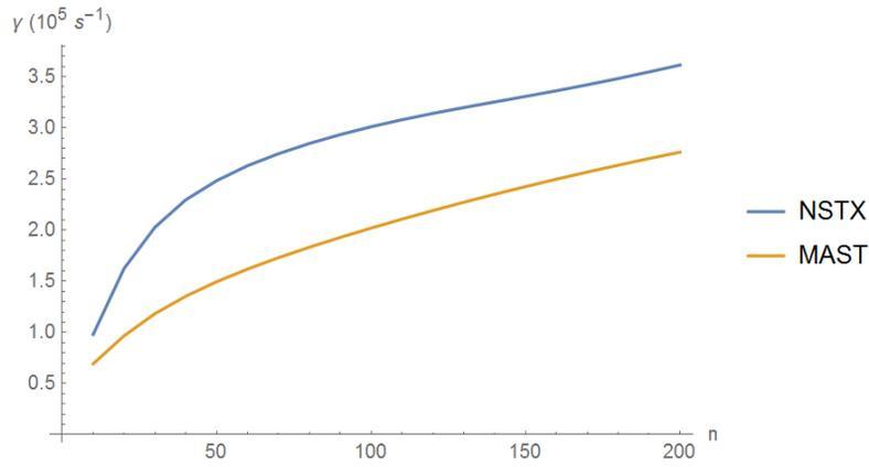
Figure 4: Growth rate as a function of toroidal mode number ( $n$ ) for NSTX and MAST-like geometries. The NSTX-like case has a density of  $n_e = 7.9 \times 10^{12} \text{ cm}^{-3}$  while the MAST-like case has a density of  $n_e = 5.31 \times 10^{12} \text{ cm}^{-3}$  at the bump peak. [Associated dataset available at <http://doi.org/10.5281/zenodo.2530371>] (Ref. 27).
