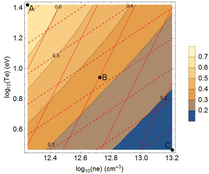
Figure 6: Color-filled contour plot of penetration ratio  $\lambda/L$  as a function of temperature and density at mode peak for toroidal mode number 100 (MAST-like geometry). See Fig. 5 for additional information and Fig. 8 for eigenmode structure. [Associated dataset available at <http://doi.org/10.5281/zenodo.2530371>] (Ref. 27).
