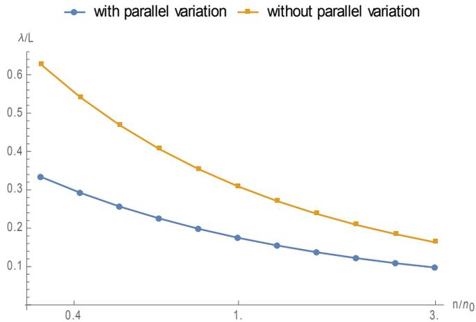
Figure 9: Penetration length as a function of relative density for case without parallel temperature variation (green) and with parallel temperature variation (blue). [Associated dataset available at <http://doi.org/10.5281/zenodo.2530371>] (Ref. 27).
