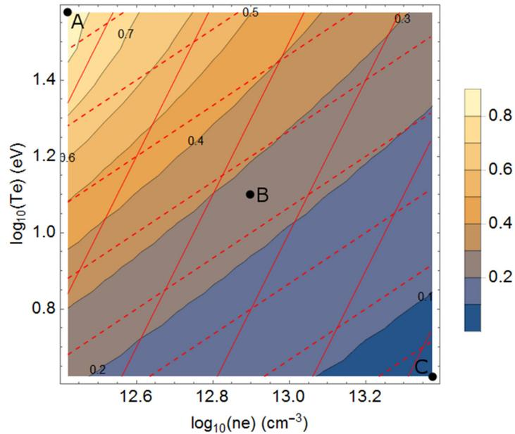
Figure 5: Color-filled contour plot of penetration ratio  $\lambda/L$  as a function of temperature and density at mode peak for toroidal mode number 100 (NSTX-like geometry). Eigenmodes for the parameters
