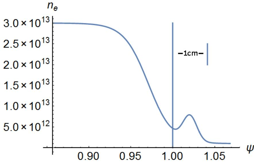
Figure 2: Density as a function of radial flux coordinate (labeled as a fraction of the poloidal flux at the magnetic separatrix) for filament simulations in MAST-like geometry. The density is taken to be a flux function in Sec. IV.B and varies along the field line in Sec IV.C (see text for details). [Associated dataset available at <http://doi.org/10.5281/zenodo.2530371>] (Ref. 27).
