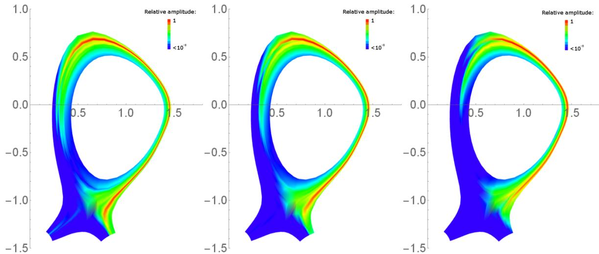
Figure 8: R-Z plots of eigenmode structure for selected MAST-like-geometry cases (left to right): Bump  $n_e=1.77 \times 10^{12}$ ,  $T_e=2.92$  eV; Bump  $n_e=5.31 \times 10^{12}$ ,  $T_e=8.77$  eV; Bump  $n_e=1.59 \times 10^{13}$ ,  $T_e=26.3$  eV. [Associated dataset available at <http://doi.org/10.5281/zenodo.2530371>] (Ref. 27).
