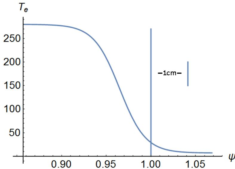
Figure 3: Temperature as a function of radial flux coordinate (labeled as a fraction of the poloidal flux at the magnetic separatrix) for filament simulations in MAST-like geometry. The temperature is taken to be a flux function in Sec. IV.B and varies along the field line in Sec IV.C (see text for details). [Associated dataset available at <http://doi.org/10.5281/zenodo.2530371>] (Ref. 27).
