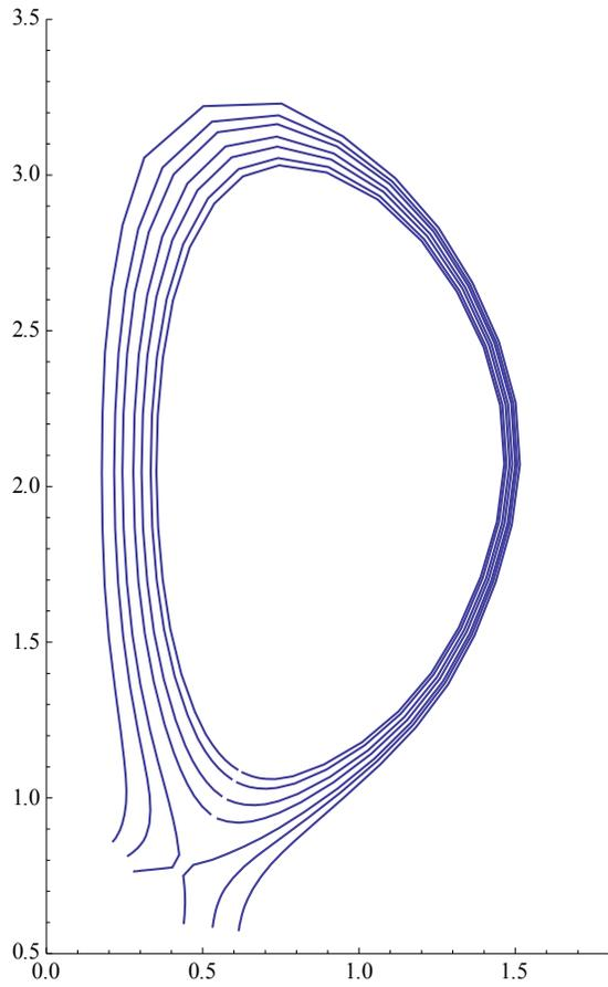
Figure 1: Sample flux surfaces for a typical NSTX-like magnetic geometry. [Associated dataset available at <http://doi.org/10.5281/zenodo.2530371>] (Ref. 27).
