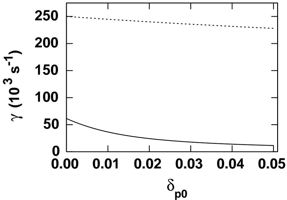
Fig. 4 Growth rate  $\gamma$  ( $10^3 \text{ s}^{-1}$ ) of the most unstable  $n = 100$  mode versus normalized neutral pressure at the divertor plate ( $\delta_{p0} = p_{0d}/p_{tu}$ ) for the field line  $\psi = 0.01$  and the high-recycling equilibrium. Shown are the ideal case (solid line) and the resistive case (dashed curve). For each curve, the most unstable value of  $\theta_0$  is independent of  $\delta_{p0}$  and has the value shown in Table II.
