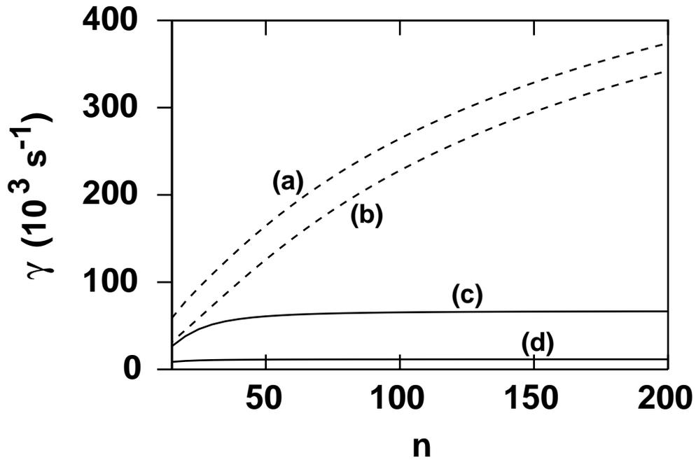
Fig. 6 Growth rate  $\gamma$  ( $10^3 \text{ s}^{-1}$ ) versus toroidal mode number  $n$  for the high-recycling equilibrium ( $\psi = 0.01$ ) with several stability models: (a) resistive model without neutrals (dashed line); (b) resistive model with neutrals (solid line); (c) ideal model without neutrals (dashed line); and (d) ideal model with neutrals (solid line). For each curve, the most unstable  $\theta_0$  for  $n = 100$  was used (see Table II).
