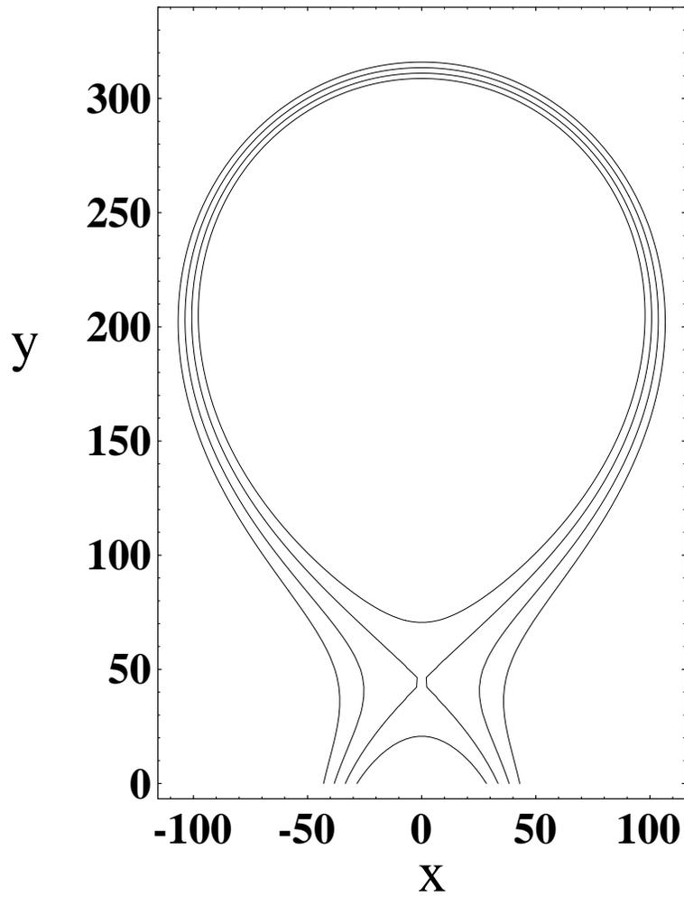
Fig. 1 Selected flux (constant  $\psi$ ) surfaces near the separatrix for the two-wire model of a single-null X-point divertor. [From Myra et al., Ref. 6]
