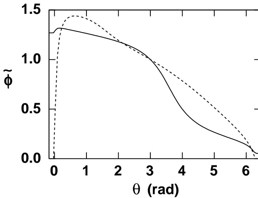
Fig. 3 Eigenfunctions  $\tilde{\phi}(\theta)$  for  $n = 100$ , the most unstable value of  $\theta_0$ , and the high-recycling equilibrium described in the text. Shown are the ideal ballooning eigenfunction with  $\theta_0 = 3.6$  (solid line) and the resistive ballooning mode with  $\theta_0 = 1.5$  (dashed line).
