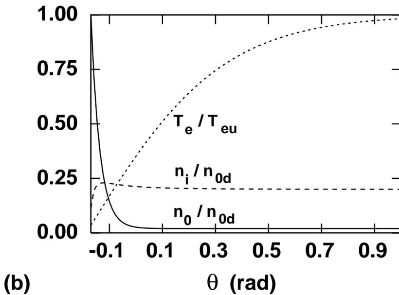
Fig. 2 Normalized equilibrium profiles  $n_i/n_{0d}$  (dashed line),  $n_0/n_{0d}$  (solid line), and  $T_e/T_{eu}$  (dotted line) versus  $\theta$  on the reference field line  $\psi = \psi_0$  for two equilibria described in the text: (a) an attached high-recycling case and (b) a detached case. Only the region near the outboard divertor and X point ( $-0.17 < \theta < 1.0$ ) is shown. The normalizations are to upstream (u) and divertor plate (d) values.
