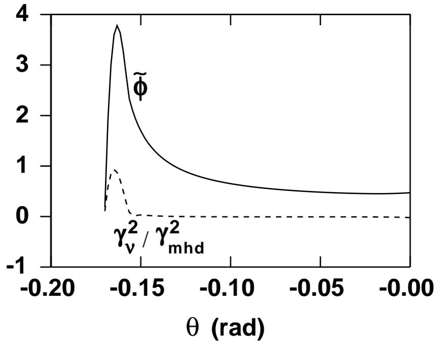
Fig. 7 Plot of the eigenfunction  $\tilde{\phi}(\theta)$  (solid line) and the instability drive  $\gamma_v^2(\theta) / \gamma_{mhd}^2$  (dashed line) in the outboard divertor region for  $n = 100$ ,  $\theta_0 = 6.3$ , and the detached equilibrium with the parameters  $T_{ed} = 0.1$  eV and  $Z_{eff} \ln \Lambda = 0.5$ . Thus, a small amount of resistivity permits a highly localized branch of the ion-neutral drag instability.
